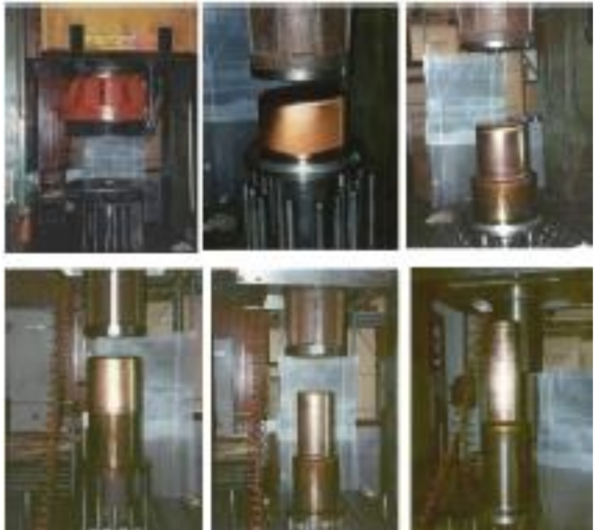
Fig. 4 – Direct Deep-Drawing of seamless tubes from circular blanks. Top picture: First drawing of a blank. Bottom picture: Redrawing of the cup into a taller one with a smaller diameter. On the left is displayed the configuration before drawing, while that on the right is during the operation.
