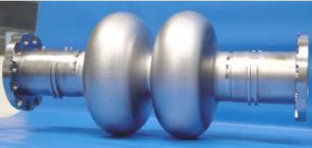
Nb bulk seamless cavity by hydroforming DESY
